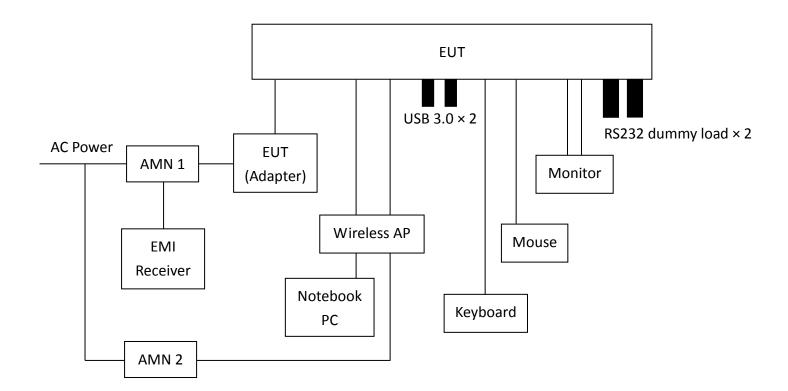
The EUT along with its peripherals were placed on a 1.0 meter(W)×1.5meter(L) and 0.8 meter in height wooden table and the EUT was adjusted to maintain a 0.4meter space from a vertical reference plane. The EUT was connected to power mains through a Artificial Mains Network (AMN), which provided 50 ohm coupling impedance for measuring instrument and the chassis ground was bounded to the horizontal ground plane of shielded room.
